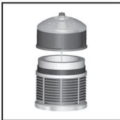
2. Return the unit to its upright position and lift off the top motor assembly.
